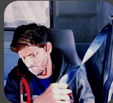
Uses marker-based detection aligned with the driver's face to ensure the seat belt is worn correctly.
