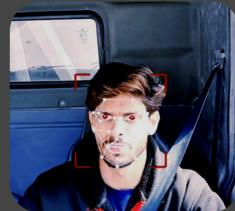
Uses facial recognition to detect driver changes in real time, alerting owners of unauthorized access.
